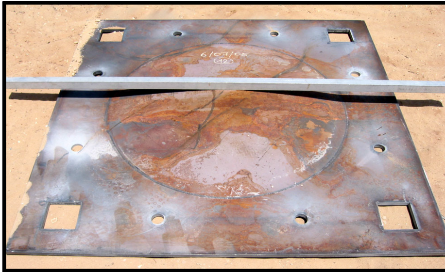
Figure 9. The final geometry of the deformed RHA plate after the experimental blast test as performed by Neuberger and his co-researchers (Neuberger et al., 2009)
