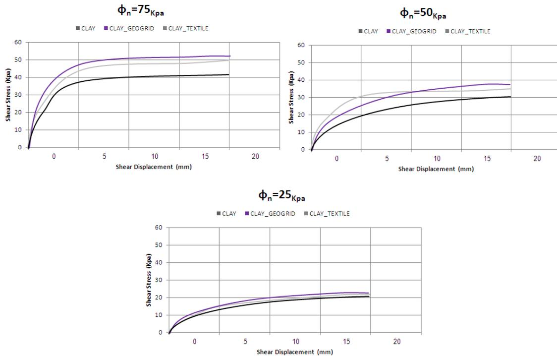
Figure 3. Shear stress curves – shear displacement of clay samples
