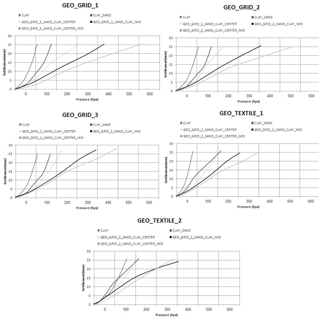
Figure 7. Pressure-settlement diagram for the reinforced samples
