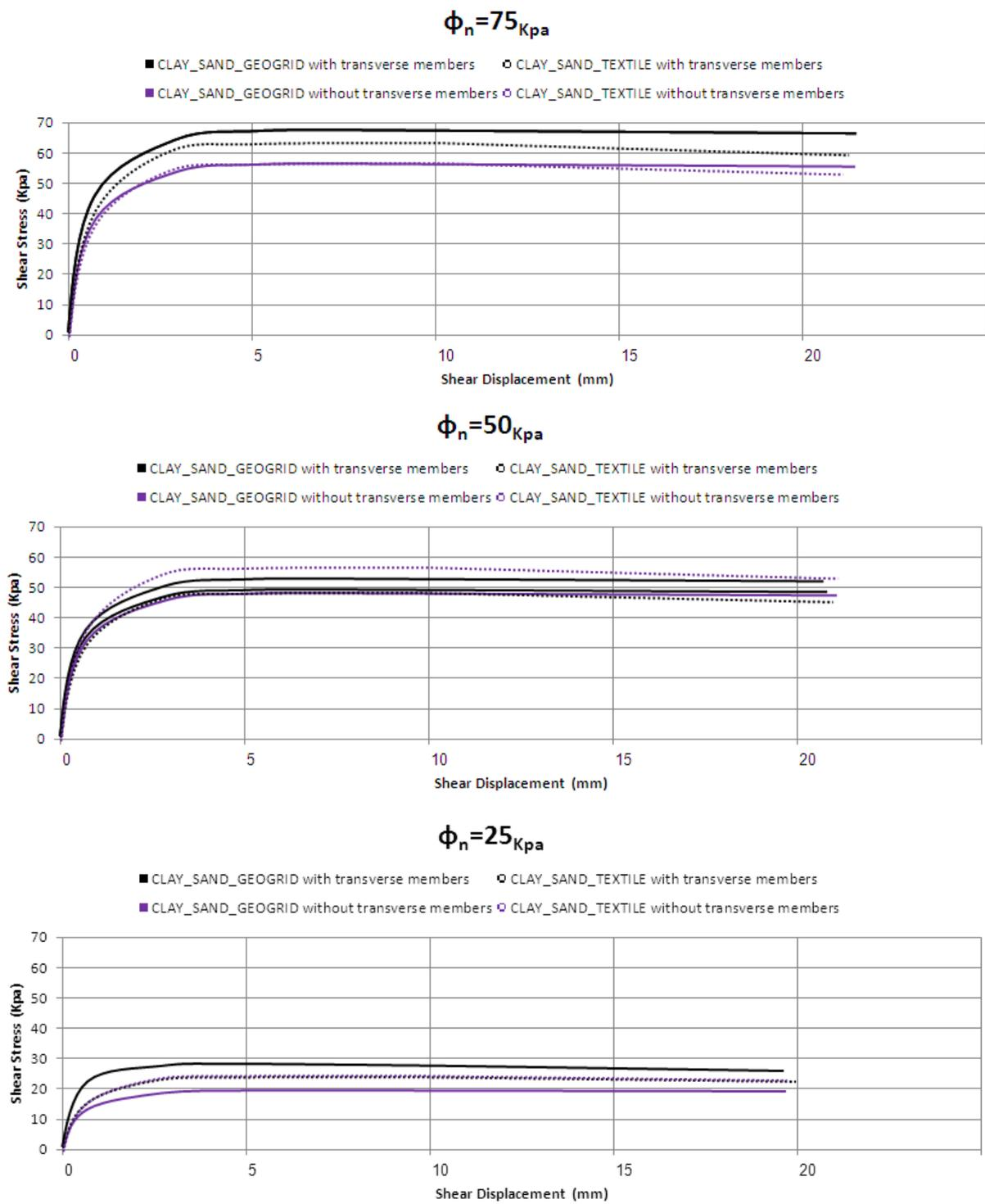
Figure 5. Shear stress-displacement curves for clay-sand-geo-synthetics samples without and without transverse members
