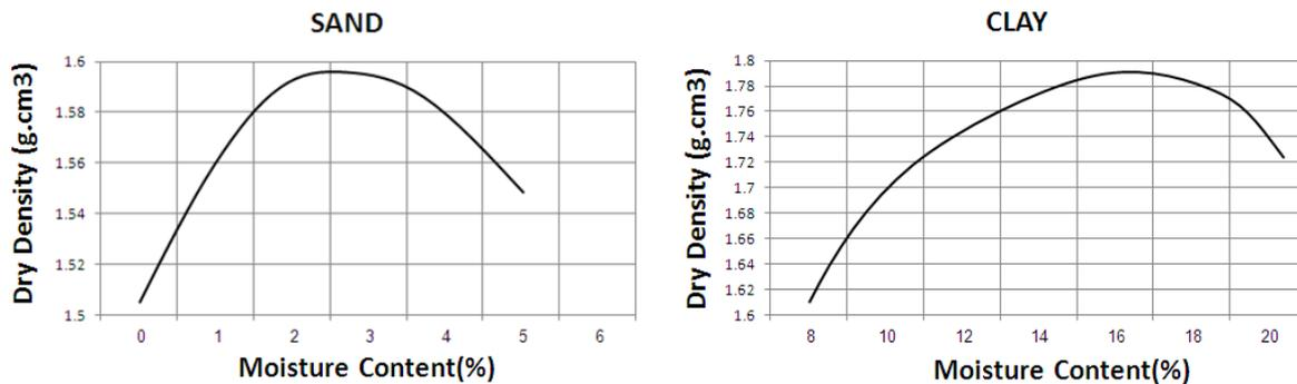
Figure 1. Clay-sand compaction curve
