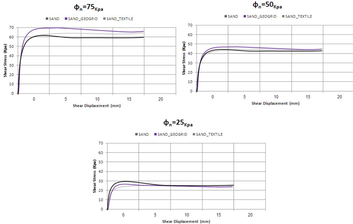
Figure 4. Shear stress-displacement curves of sand samples
