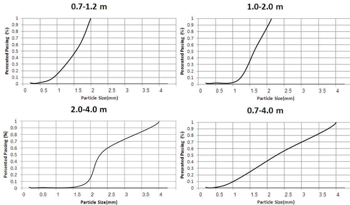
Figure 2. Sand gradation curve
