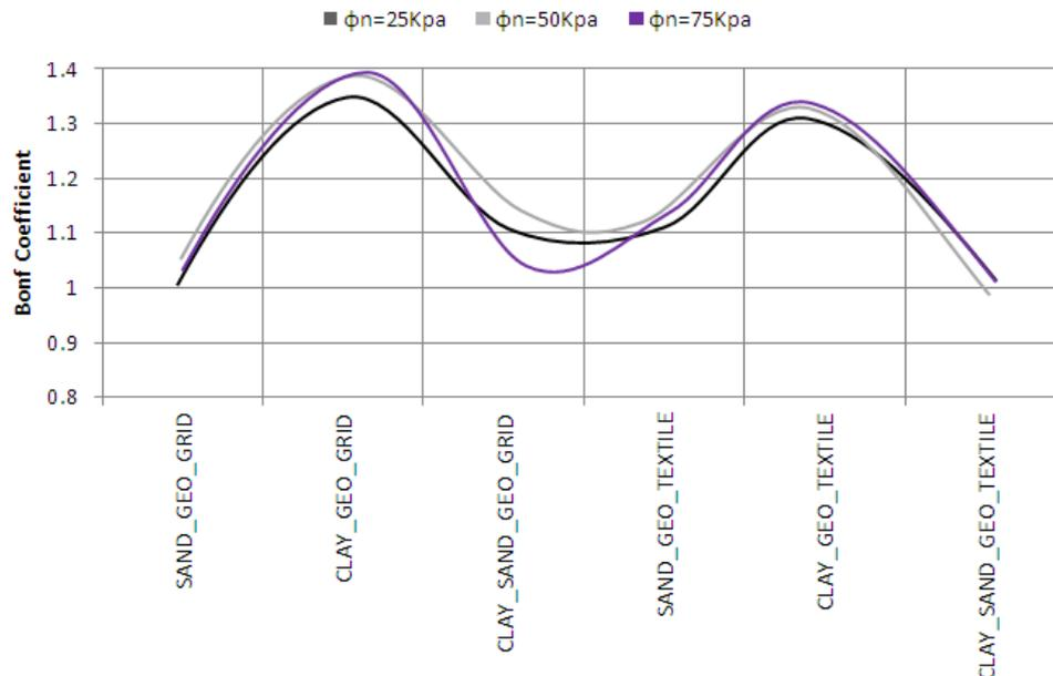
Figure 6. Bond coefficient changes of geo-synthetics compared to vertical stress
