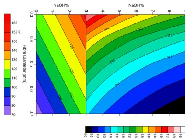
Figure 5. Contour graph for fibre diameter-NaOH%-UTS relationship
