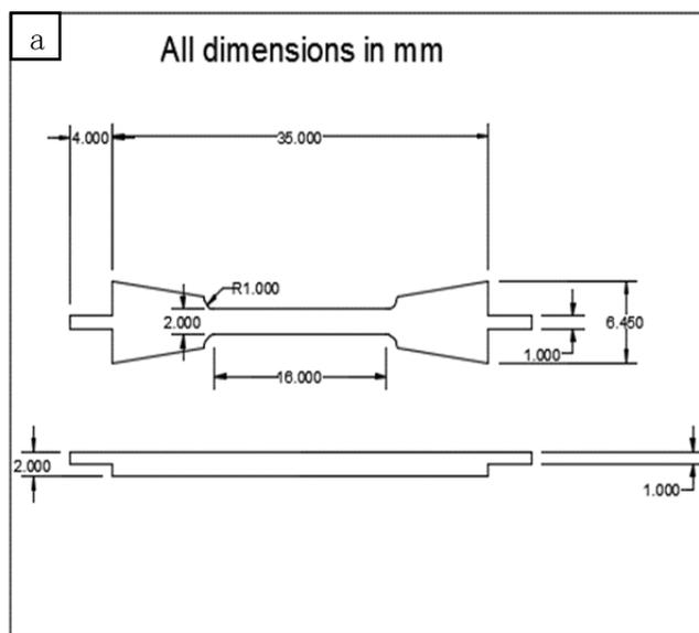
Figure 2.a The specimen geometry
