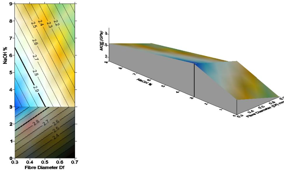
Figure 7. Response surface and Contour Graph for fibre diameter-NaOH%-MOE
