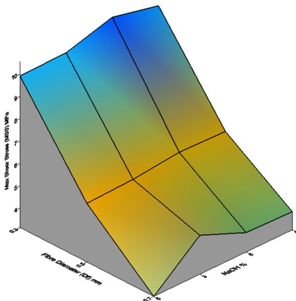
Figure 11. Surface representations for MSS-NaOH%-Df experimental results
