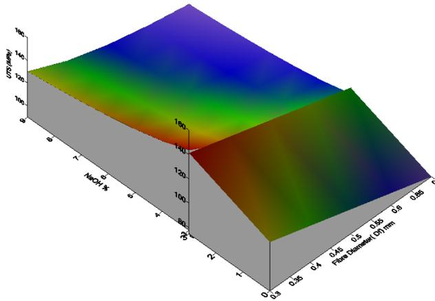
Figure 4. Three-dimensional surface for fibre diameter-NaOH%-UTS relationship
