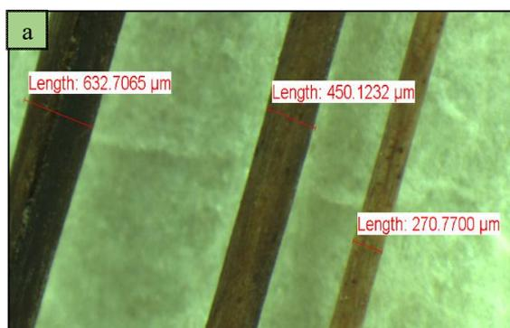
Figure 1.a Diameter measuring using OM
