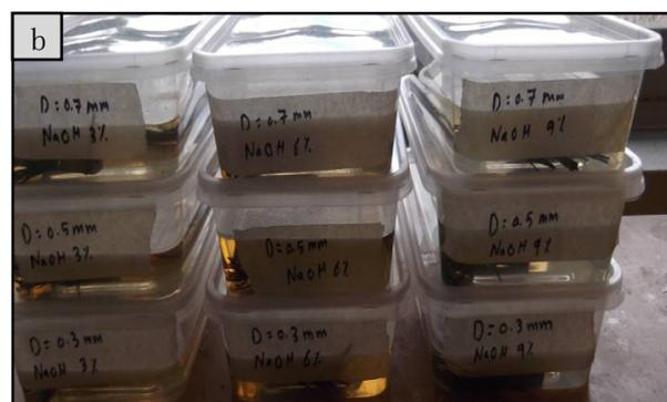
Figure 1.b Fibre treatment using NaOH solution
