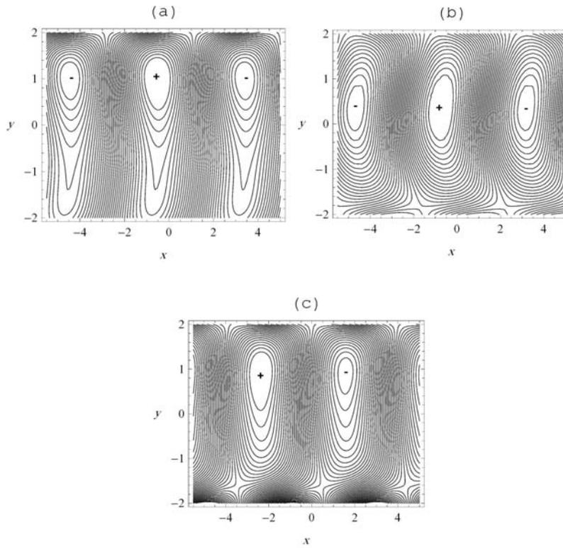
Figure 2. Streamlines contours for a system having the parameters  $V_{01} = 4, V_{02} = 1, H_{01} = 2, \hat{\mu}_1 = 0.7, L_1 = 0.6, L_2 = 0.9, \hat{\rho}_1 = 0.9, \hat{\rho}_2 = 0.7, Q_1 = 0.5, Q_2 = 0.3, Q_3 = 0.5, k = 0.3$  and  $t = 0.2$ , while  $\hat{\mu}_2 = 0.2, 0.5$  and  $0.7$  of the parts (a), (b) and (c), respectively.
