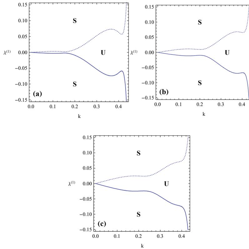
Figure 4. Illustrated in the plane  $(\lambda^{(1)} - k)$  according to equations (42), for a system having  $V_{01} = 4, V_{02} = 1, H_{01}=2, \hat{\mu}_1 = 0.2, \hat{\mu}_2 = 0.7, L_1 = 0.6, L_2 = 0.9, \hat{\rho}_1 = 0.9, \hat{\rho}_2 = 0.7, Q_1 = 0.5, Q_2 = 0.3, Q_3 = 0.5$ , with  $V_{02} = 2, 5$  and  $7$  of the partitions (a), (b) and (c), respectively.
