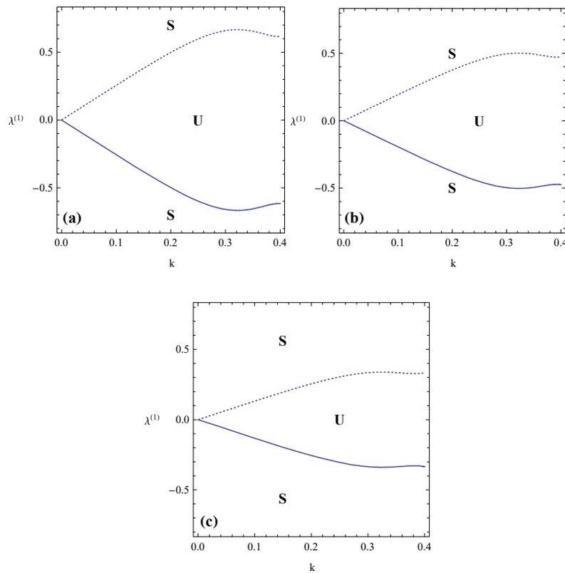
Figure 6. The stability diagrams in the  $(\lambda^{(1)} - k)$ , with the same parameters given in Fig. 4 at  $H_{01} = 10, 20$  and  $30$  of the partitions (a), (b) and (c), respectively.
