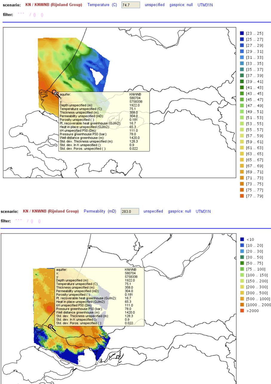
Figure 5. Temperature and permeability distribution in KN aquifer area
