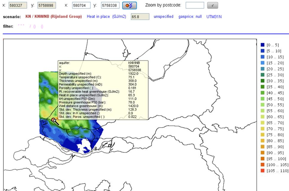
Figure 4. Heats in place, aquifer group KN, KNWNB type
