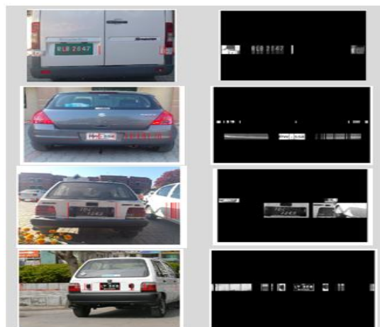
Figure 8. Outputs of horizontal projection
