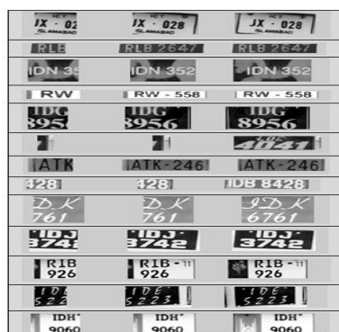
Figure 9. Results of growing window stages performed on different registration plates
