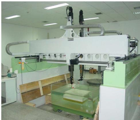
Figure 5. The seismic data acquisition system in CNPC key lab
