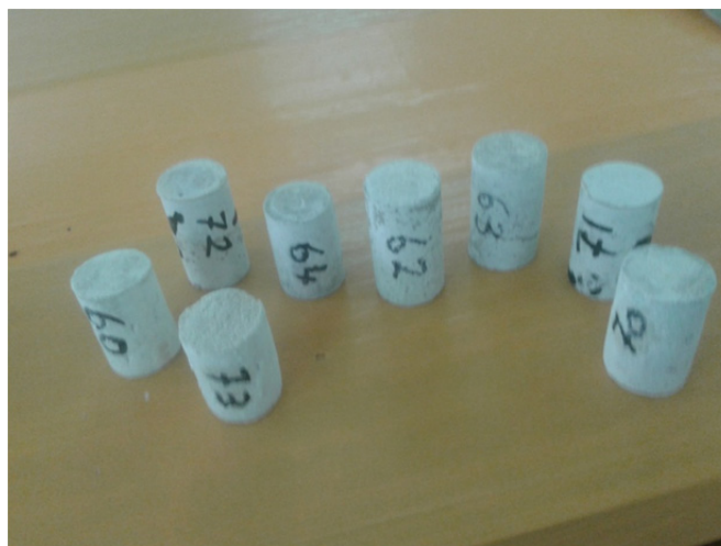
Figure 3. Fluorescence phenomena on NaOH- metakaolin mixtures
