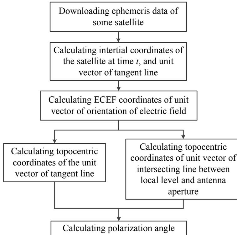
Figure 2. The calculation flow of polarization angle
