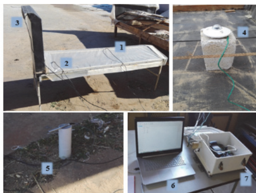
Figure 1. Experimental set-up of the solar tunnel dryer and the equipment
