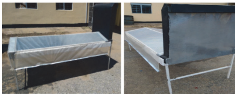
Figure 2. Side and rear views of a solar tunnel dryer
